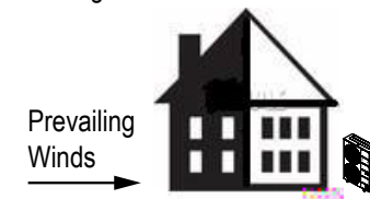
Figure 35: Leeward Side of the Building.
