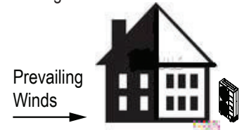
Figure 40: Leeward Side of the Building.
