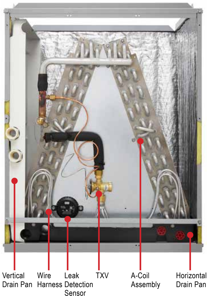
Figure 3: A-Coil Components.
