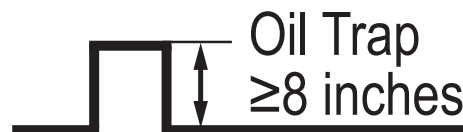
Figure 59: Close Up of An Inverted Oil Trap.
