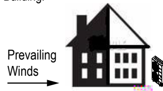
Figure 43: Leeward Side of the Building.
