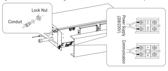
Figure 31: Close Up of Heat Recovery Unit Terminal Block.
