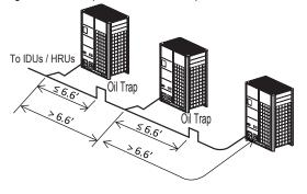
Figure 43: Inverted Trap Applications.
