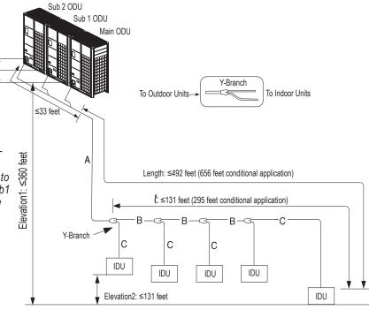
Table 26: Main Pipe (A) Diameters from Outdoor Unit to First Y-branch / Header Branch.
