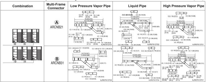
\*For example, the indicated Ø3/8 (9.52) is the outside diameter (O.D.) of the field-joined piping. MEZ62225512 4/18/2017
