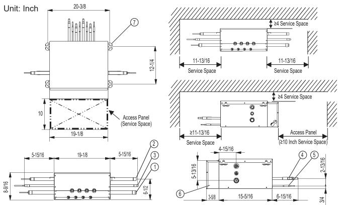
Table 35: PRHR023A to 043A Heat Recovery Unit Components.
