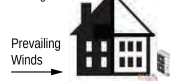
Figure 52: Leeward Side of the Building.
