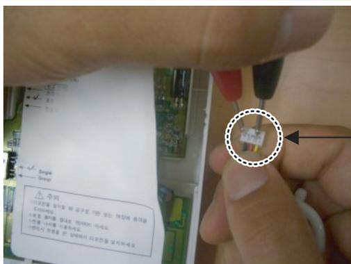
Checking communication cable connection status
