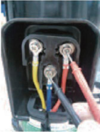
\* Measuring input voltage
