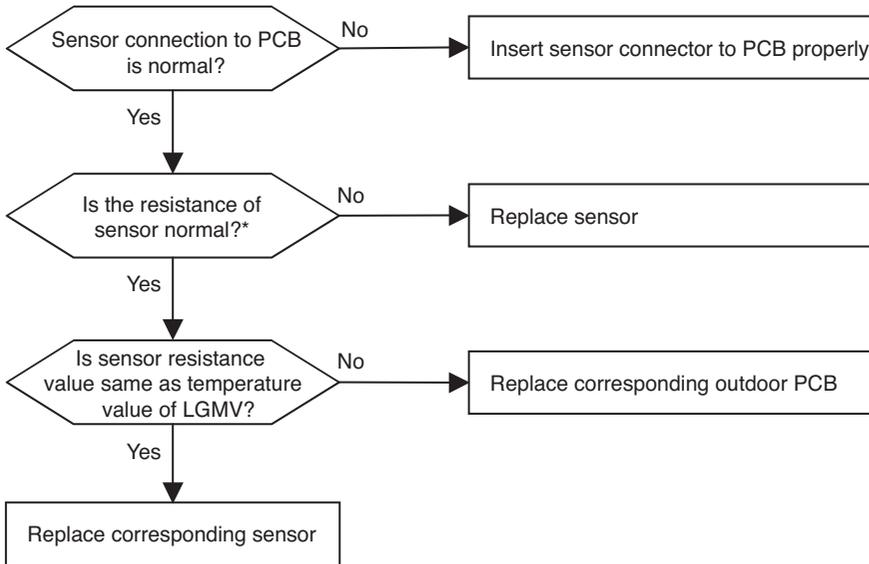
\* Error is generated if the resistance is more than 5 M(open) and less than 2 k (short)
