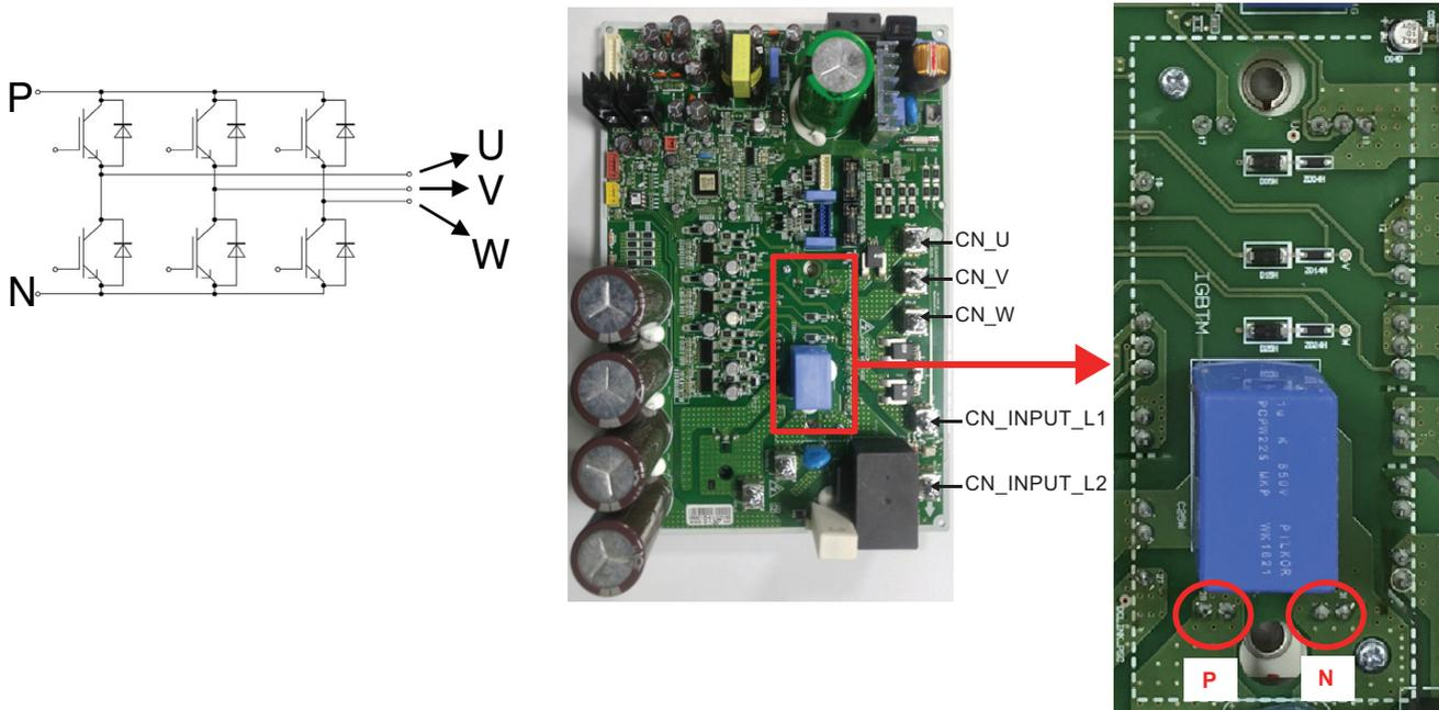
1. Wait until Comp PCB DC voltage gets discharged, after the main power switch off (10 minutes).
