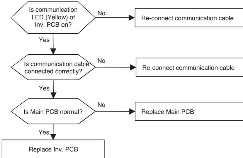
\* The method of checking Main PCB and Inv. PCB (If normal, communication LED blinks)
