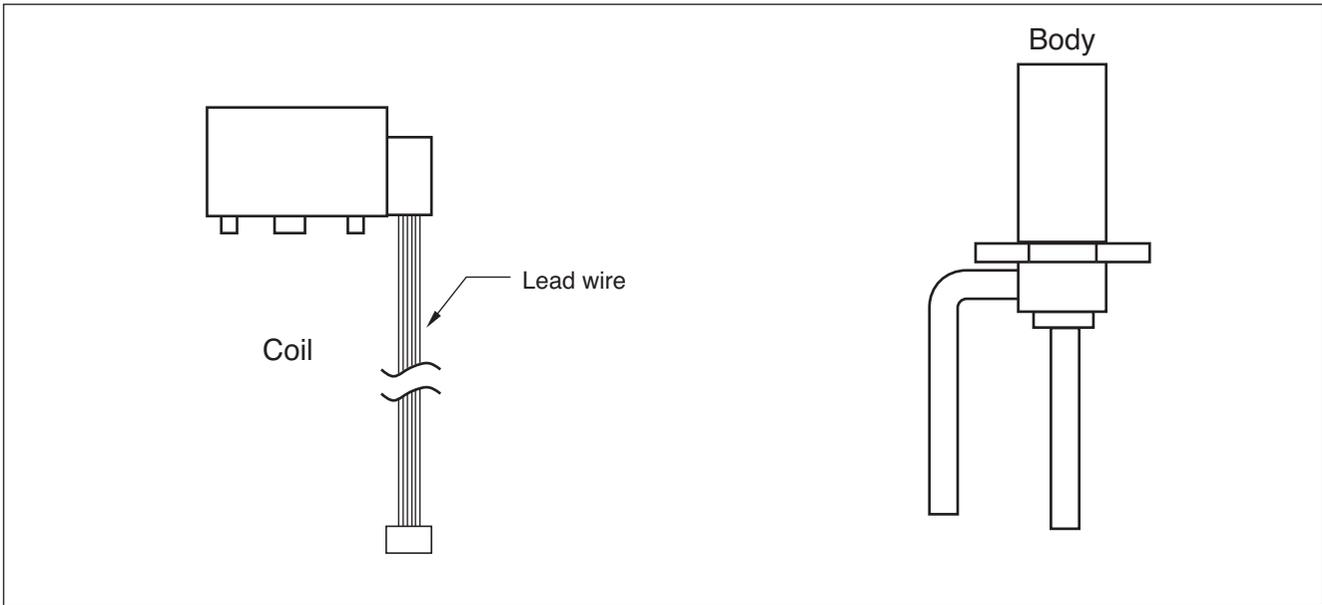
• Remove and assemble the coil
