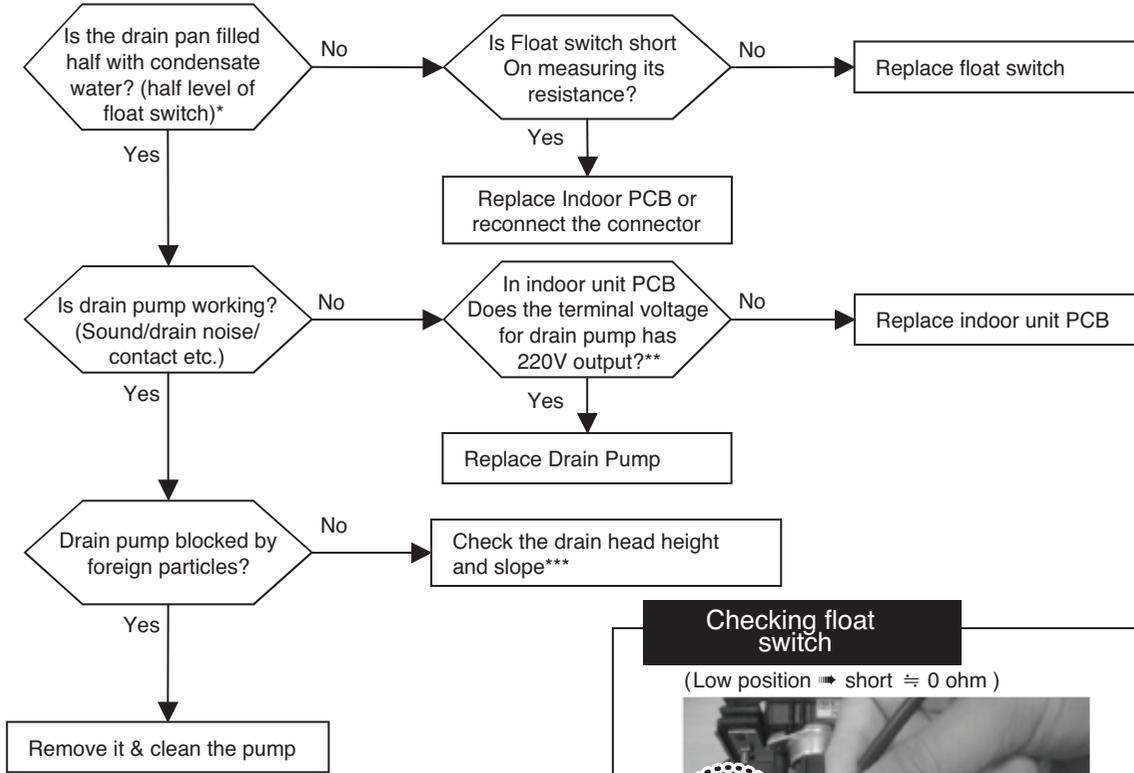
\* If the float goes up higher than a half of float switch then the circuit is open & the unit is stopped automatically.
