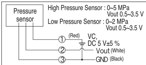
The pressure sensor is composed like the circuit picture shown above. If DC 5 V voltage flows on red and black wire, voltage would be made between the white and black wire. The pressure which is equivalent to the pressure output is shown in the table above.
