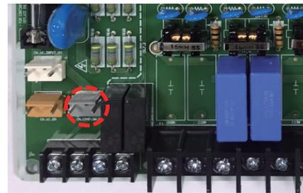
Note 2) Check short with high pressure switch connector
