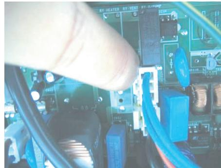
\*\*\* Indoor PCB drain pump connector
