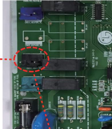
\*\* Confirm the 4way valve coil is inserted to the end
