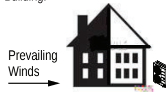
Figure 26: Leeward Side of the Building.
