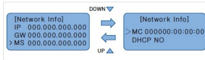
To change the network setting, locate the arrow on the corresponding setting position and press **[SET]** button to enter the corresponding setting screen.
