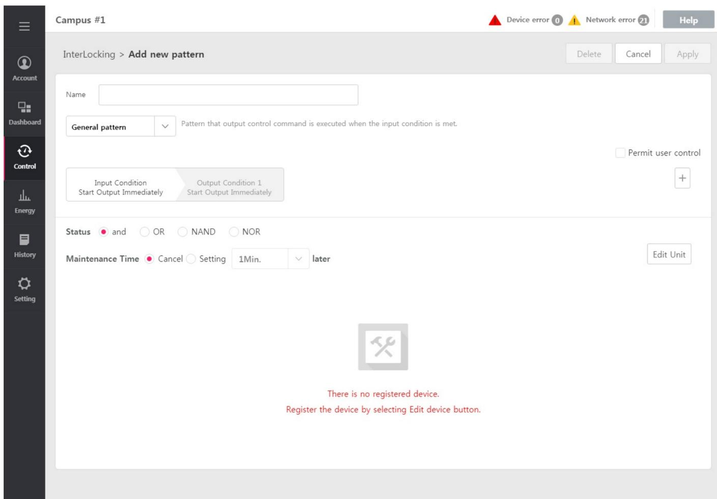
3. In the InterLocking name input field, input the desired InterLocking name.
