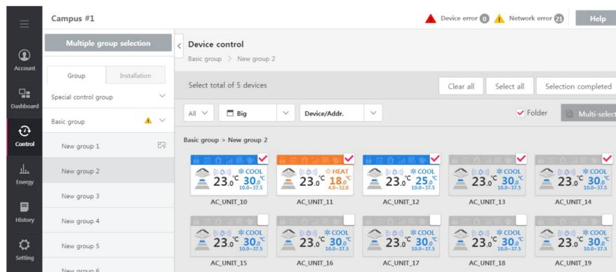
5. In the control window, set the corresponding equipment's control status.
