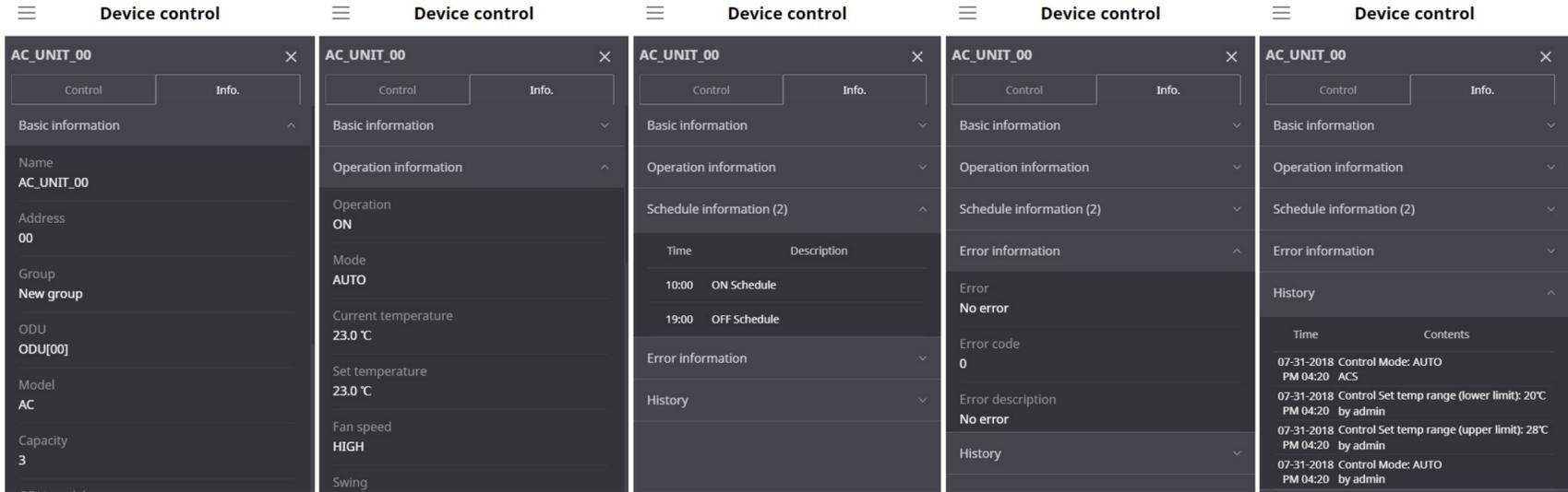
The image displays five sequential screenshots of the 'Device control' interface for a device named 'AC\_UNIT\_00'. Each screenshot shows a different tab selected in the 'Info.' section.
