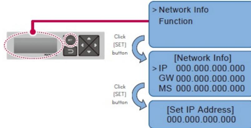
2. While IP is selected, if you press **[SET]** button, screen to input IP address is displayed.
