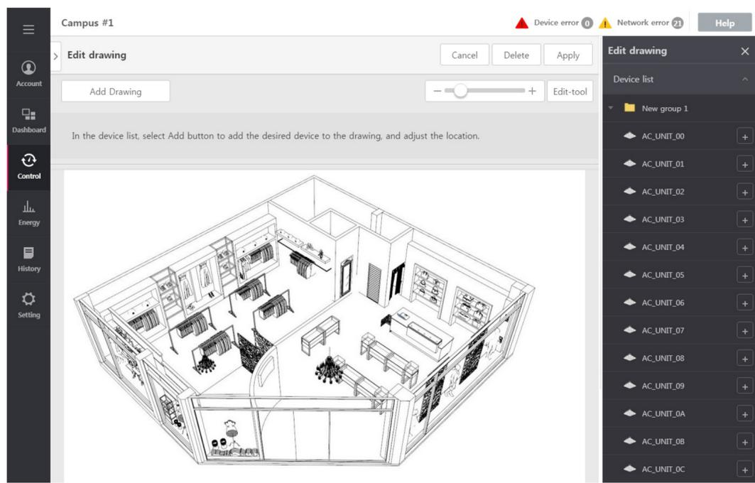
7. To add device in the drawing, select the desired device in the device list in the right side Edit drawing window, and click [+] button. The device is added in the drawing section.
