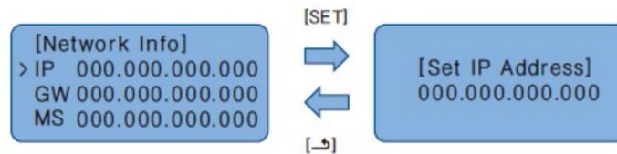
The network address consists of four 3-digit numbers. In case of setting the network address, the name of the related address is displayed on the LCD of ACP 5, and you need to press **[▲]**, **[▼]**, **[◀]**, **[▶]** button for the setting.
